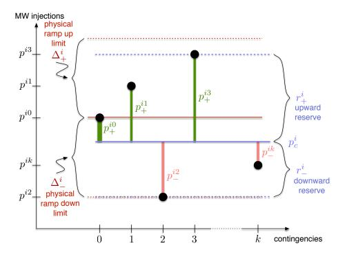
Figure 3-3: Reserve Structure for Generator i
