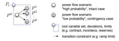
Figure 3-2: Secure Dispatch Problem Structure
